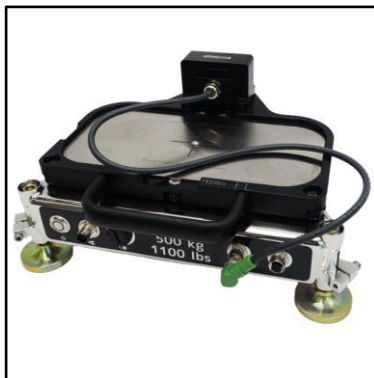
Platform calibration frame and camber sensor (inclinometer)
